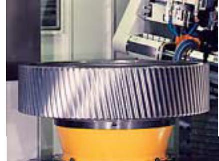
Helical Gear Grinding
